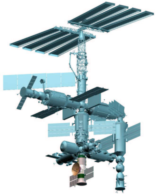
Figure 2. Submillimetron module docked to Russian Segment of the ISS for service and instruments replacement. Observational phase begins after screens deployment and detachment from ISS
